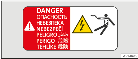
Fig. 4 Warning sign on high-voltage components.
