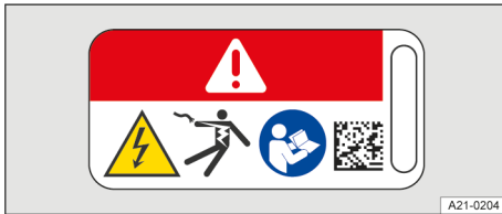
Fig. 5 Warning sign on high-voltage components.
